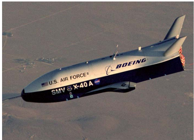
Figure 1. Boeing’s X-40A RLV in Drop Tests.
